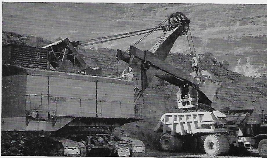
Below, shovels mine the ore from the pit bottom. The rock-over skip system, right, when completed, will lift all ore and waste rock out of the pit.
